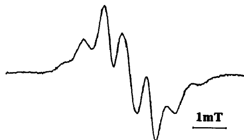
Figure 2. ESR spectrum of 3 in the solid state under UV irradiation at -100°C.
